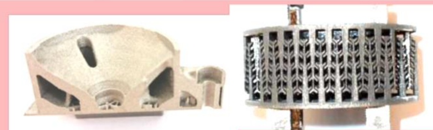
Base plate and flexible thermal structure made of ALSi10Mg, Mašek 2022
